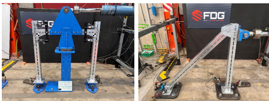
Figure 1 - Modframe cyclic test typical setup - portal frame (left) and braced cantilever (right) tests
